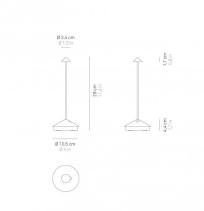
Pina pro is a rechargeable table lamp, with contact charging base, painted aluminum body, polycarbonate diffuser and LED light source. It is equipped with a dimmer touch control and has an IP65 degree of protection which makes it suitable for both indoor and outdoor use.
