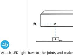
sure they are fully inserted with no gaps. Ensure each joint is positioned so that the joint's center opening is always facing inward, and not upward, downward or outward of the entire fixture.
