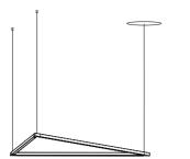
There are two ways to mount the Z-Bar pendant triangle, a monopoint installation or a multipoint installation. For monopoint installation, proceed to step 2. For multipoint, see below.
