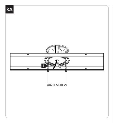
1 Attach the mounting plate to the electrical box using the two #8-32 screws provided.
