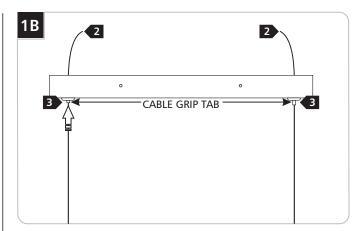
**NOTE:** When cutting the support cable to desired length, leave extra cable for fine tune leveling.
