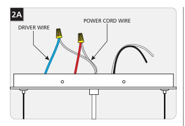
1 Take note of the wire connections and remove the wire nuts to disconnect the power cord wires from the driver wires.
