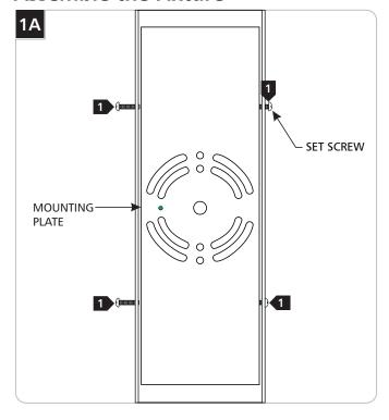
1 Unscrew the four set screws from the canopy and remove the mounting plate.
