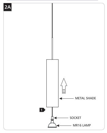
1 Move the fixture metal shade up to expose the socket.
