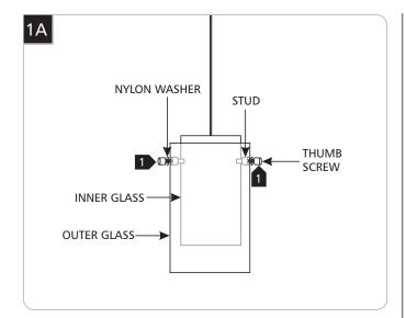
1 Line up the outer glass holes with the inner glass studs and secure the outer glass to inner glass with provided thumb screws and nylon washers.
