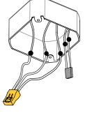
Screw backplate in junction box with screw 2x 8-32 machine screws (not included)
