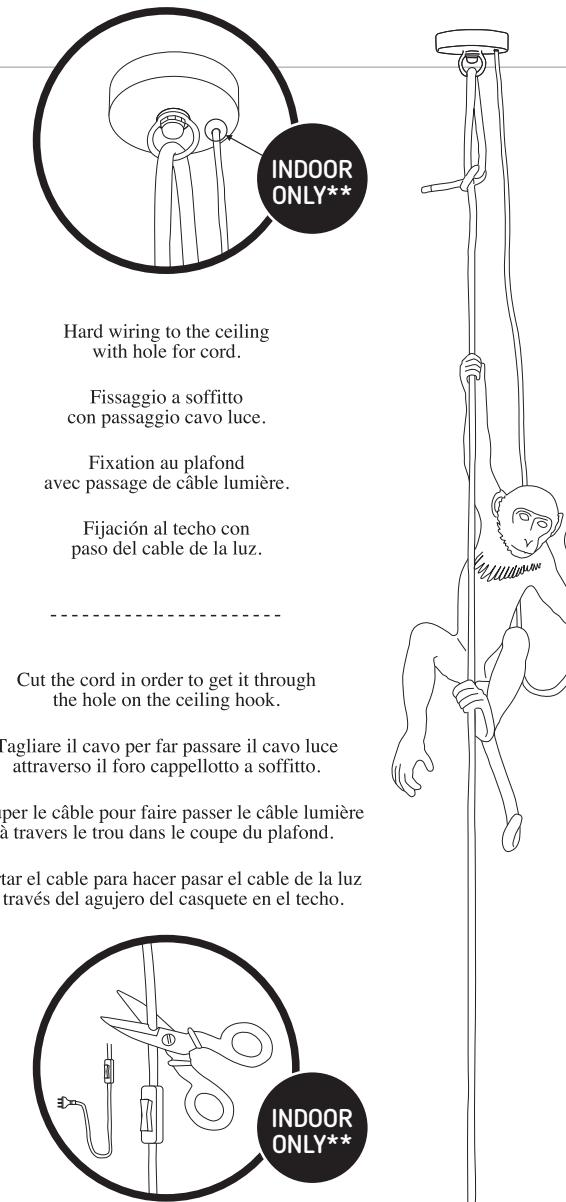
Hard wiring to the ceiling
