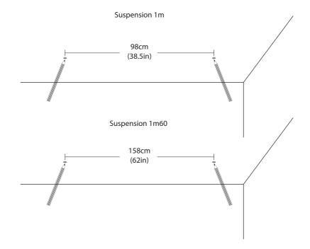
2) Fix the anchors with appropriate screws
