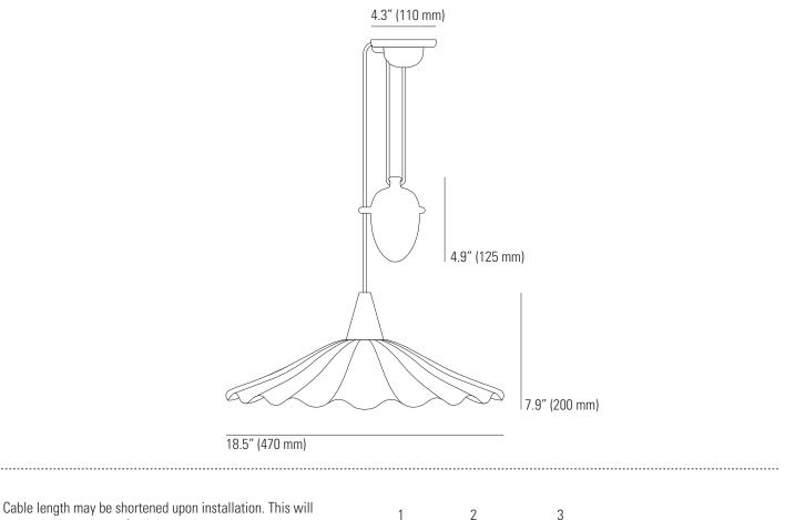
Cable length may be shortened upon installation. This will reduce both maximum & minimum dropand reduce the range of movement.
