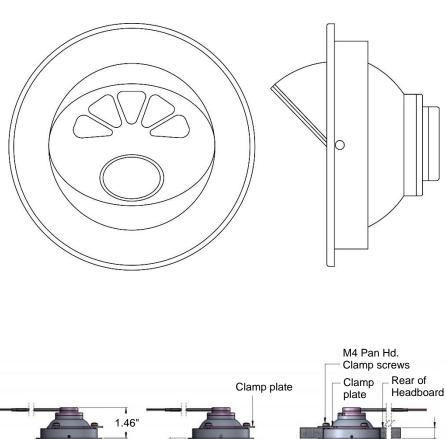
0.47" min Ø 2.75" RECOMMENDED APERTURE to 1.57" max LIGHT ON FOR INSTALLATION Headboard **Dimensions in inches** Dimensions in inches Thk
