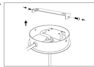
Attach the ceiling plate to the bracket with the screws.
