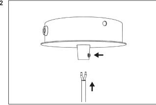
Lead the fabric cable in through the cable relief at the bottom of the ceiling plate.
