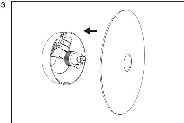
Carefully place the cover plate over the socket.
