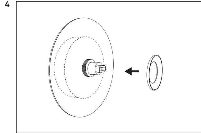
Carefully place the small metal plate over the socket.
