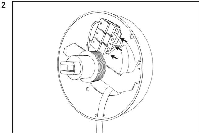
Lead the power cable in through either the bottom or the back of the ceiling plate
