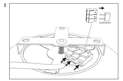
Install the power cable by leading it into the cable connector.
