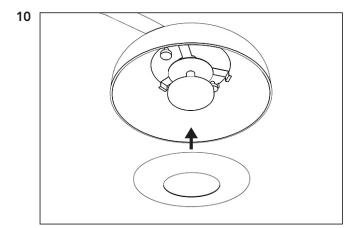
Attach the inner plate by carefully sliding it up and let the magnets fixate the plate to the lamp.
