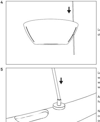
Lead the wires through the top of the cover plate.
