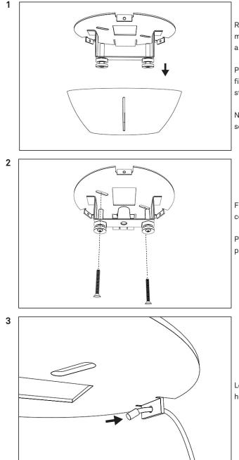
Remove the cover plate from the mounting plate by pulling them apart by hand.
