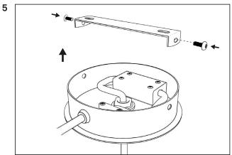
Attach the ceiling plate to the bracket with the screws.
