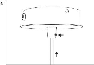
Adjust the lenght of the fabric cable to fit your specifications.
