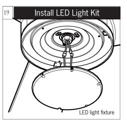
Connect white wire from fan to white wire from LED light fixture and then connect blue (or black) wire from fan to blue (or black) wire from LED light kit.
