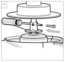
Helpful hint: For easy assembling of the cross pin on the next installation step. After slip downrod into the motor yoke, carefully insert a Phillips screwdriver through the yoke and downrod (don't damage the lead wires) as a guide and then push the cross pin and pull the screwdriver in the meantime as shown in the illustration.
