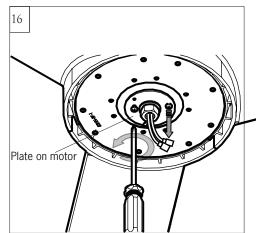
Loosen 2 and remove 1 preassembled screw from the plate on motor. Save screw for later use.
