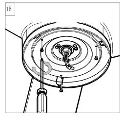
Remove 3 preassembled screws from light pan. Keep screws.
