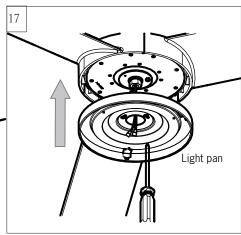
Place light pan over the lead wires and attach it onto the plate on motor, aligning the keyhole slots on the light pan with the preassembled screws on the plate. Twist clockwise till lock.
