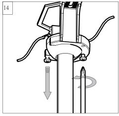
Partially loosen one and remove one preassembled screw from mounting bracket. Save screw.
