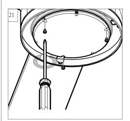
Attach LED light kit onto the light pan, aligning the holes on the LED light kit with the screw holes on light pan. Reinstall the screws removed in step 19. Tighten all screws securely.
