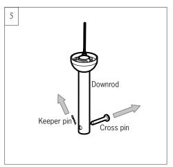
Remove preassembled keeper pin and cross pin from downrod. Keep parts.
