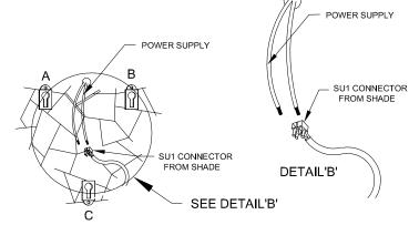
2. Connect the flat cord to the power supply w/ the SU1 connector.
