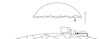
Remove the allen wrench and pull KRIS KROS wall lamp cap apart.
