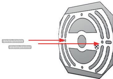
**3** First, connect the ground to the green screw on the mounting plate.
