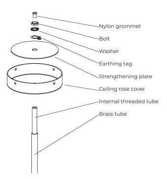
**1**. Fix the mounting plate to the ceiling. Ensure that suitable screws are being used for the surface that you are mounting to (not supplied) .
