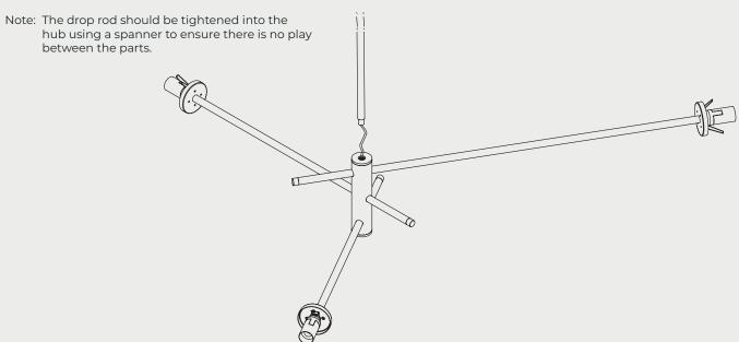
Raise the pendant and make the electrical connections ensuring all wires are colour matched and the pendant is earthed correctly.
