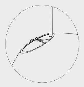
d. Once all the arms of the bracket are in the glass shade, fix the position of the glass opening using the locating ears, allowing the shade to rest on the buffers.
