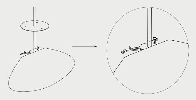
c. By keeping the lip of the glass as close as possible to the drop rod, rotate the shade while fitting each bracket at a time.
