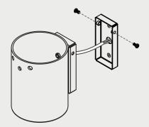
**4**. Attach the glass mounting bracket to the body with the provided M5 bolt using an allen key.
