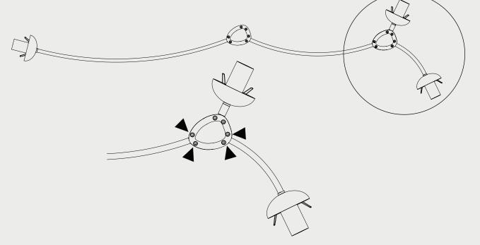
2. C. Gently turn the parts so the arrow stickers on the arm and the arrow stickers on the hub align. D. Tighten the loossed screws securing the parts in place. E. Tighten all 6 screws on the hub and repeat several times until all screws are well tighten and fully secure. Ø) 0 6
