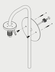
1. For US installation, fit the supplied US adapter plate to the junction box using suitable screws.
