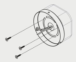
2. Raise the fitting towards the mounted wall plate and make the electrical connection.
