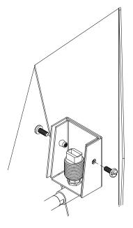
Attach the Abstract to the wall bracket, securely put the screws into place.
