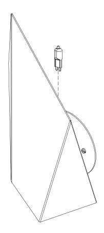
Gently push the G9 halogen bulb into the lampholder, we do not supply the bulb.
