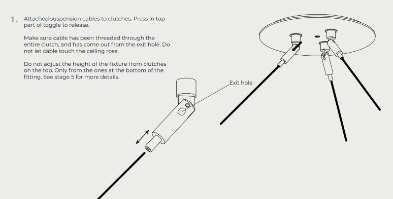
Install fitting body, with the cover plate already on top in place, make sure to align positive (+) clutch to positive clutch and negative (-) to negative. Each clutch will be marked with a small removable label.
