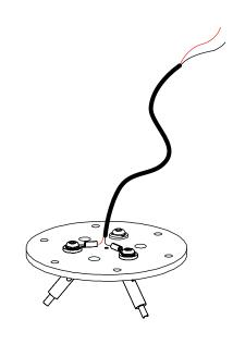
Mark out fixing hole, and use suitable fixings for the fittings weight. x6
