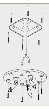
4. Attach to ceiling and install cover plate, with M3 screw.
