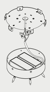
**3** Bring the ceiling rose cover up to the mounted plate and secure with the six screws.
