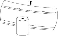
Set to correct desired height, make sure fitting is level using a spirit level. Critical, do not let fitting hang unbalanced. Make note of minimum height of fitting.
