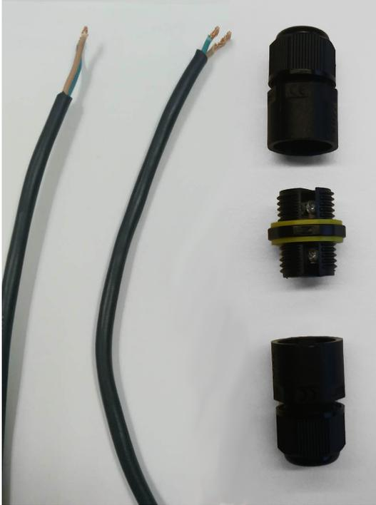
1. Prepare terminal connector and 2 wires, remove 0.8 inches sheath (X) and remove 0.4 inches jacket (Y).
