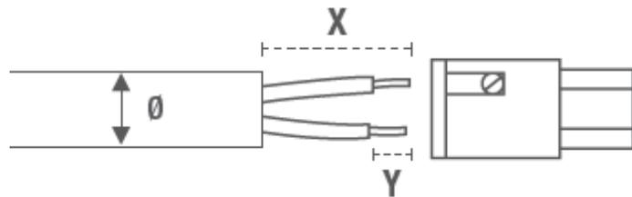
2. Back out the screws in the terminal block a little to ensure following easy connection.
