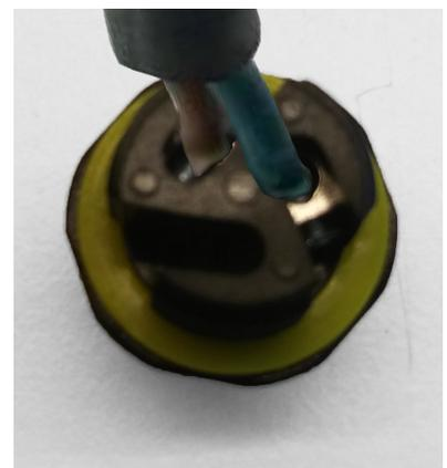
3. Plug the wires into the terminal block and screw tighten, make sure that the color of wires should be correspondingly.
