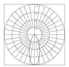
Maximum Candela = 736 Located at Horizontal Angle = 0, Vertical Angle = 0
