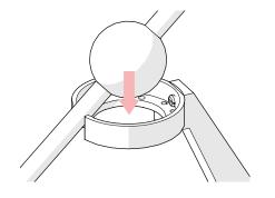
Sliding the arm through the slot in the top cap replace top cap.
