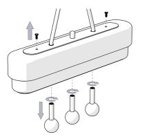
Remove glass shade by raising one end of glass and brass plate, sliding opposite end off mounting plate, then entire glass shade down assembly.
