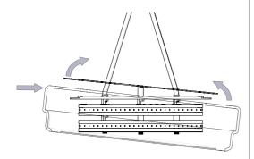
Replace 2x screws into top of fixture and tighten gently, marble orbs and rods to bottom of fixture.
