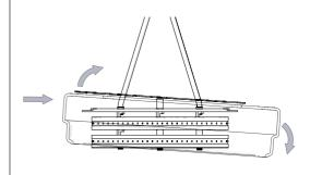
Disconnect electrical connectors and remove unwanted LED tape by carefully peeling off aluminium mounting block.
