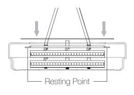
Replace 2x screws into top of fixture and tighten gently, marble orbs and rods to bottom of fixture.
