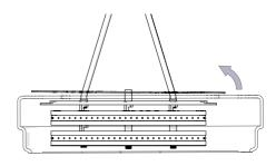
Carefully rest shade onto aluminium mounting plate, ensuring it sits flat and in-line with resting points.
