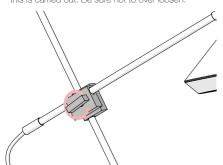
Adjust the angle of the arms of the shade as desired and then retighten the blocks.
