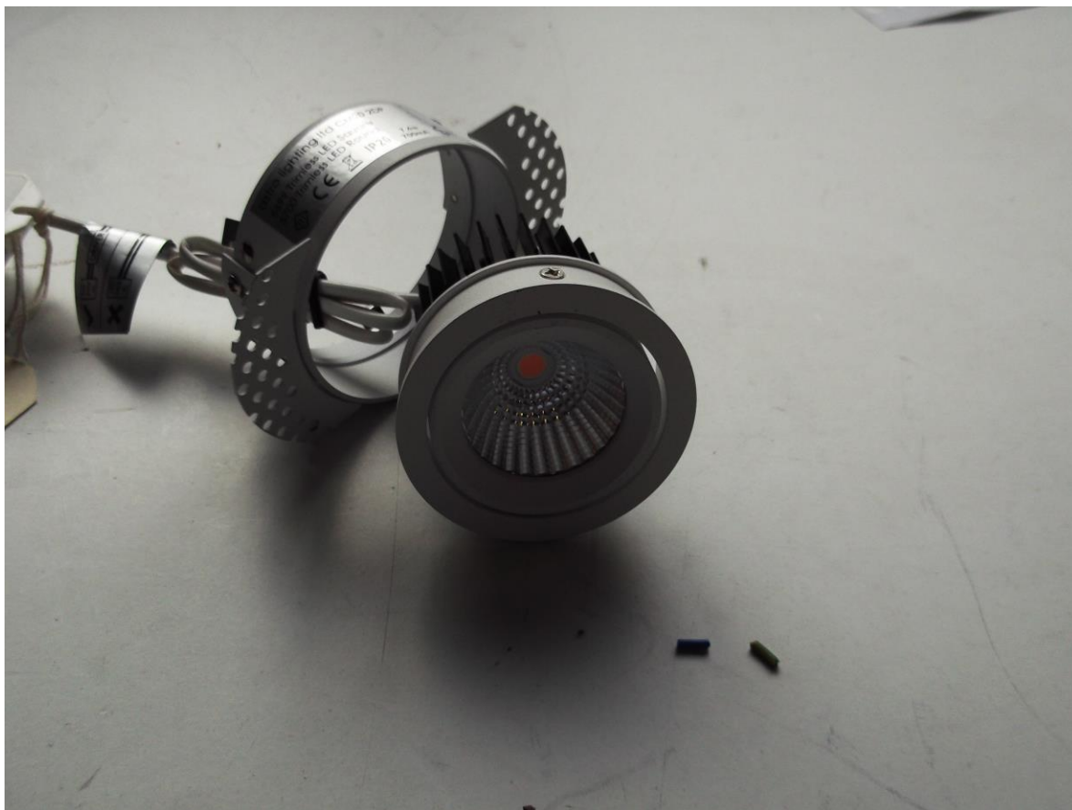
Photo 1: Luminaire on goniometer mount
