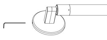
Push electrical connections into J-box and secure fixture to mounting plate with (2) set screws.
