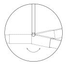
All Bough fixtures feature a 0–15° adjustable ball swivel that allows fixtures to be configured in different angles.
