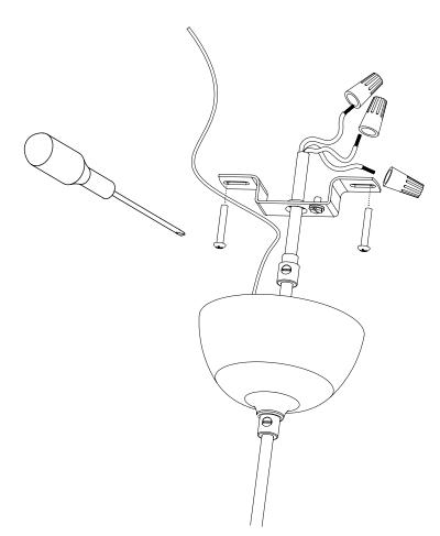
Connect wires to power cables and connect the grounding  $\quad$  Push canopy up and tighten the screw. wire to bracket.
