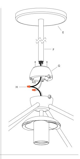
9. Secure the two half hubs together using a hex key and the provided #8-32 socket screws on either side.
