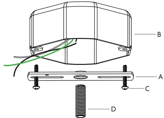
2. Cut the electrical cable to desired length and feed through the bushing in the ceiling canopy (E) and the nipple.
