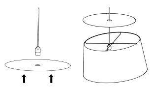
Following shade and top diffuser installation, install light bulb into socket.
