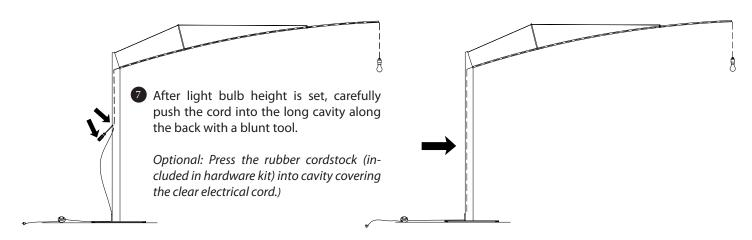
(Stretching the rubber cord can make it easier to press into the cavity, but will effect its overall length. Excess rubber cord can be trimmed easily with scissors.)
