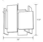
Dimensions: 15" Ø, 11.5" Materials: solid wood, polymer Product weight: 7 lb Light source: integrated LED Light output: 1250 Lumens (source) Light color: 2700 K or 3500 K Color accuracy: 90+ CRI Power usage: 13 W Dimmable (see driver below) White (CM-060) extended-profile round canopy with white braided cord and steel cable included Canopy dimensions: 5.5"Ø, 2" Canopy required to house LED driver (3.3" x 1.6" x 1.0") See website for more canopy information 72" drop length, field adjustable
